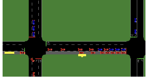
Fig. 4: Illustration of the SUMO simulation environment, where the bus is depicted in yellow, CAVs are shown in red, and HVs are shown in blue. DLs are highlighted in grey, with bus stops marked in yellow.
